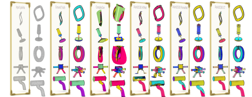
Columns: 1. input point cloud, 2. ground truth mesh, 3. reconstruction by ComplexGen, 4. HPNet segmentation + Point2CAD, 5. ParSeNet segmentation + Point2CAD, 6. GT segmentation + Point2CAD.
